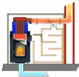
Boiler operation with Moritz's flap
