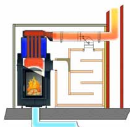
Boiler operation with Moritz's flap
