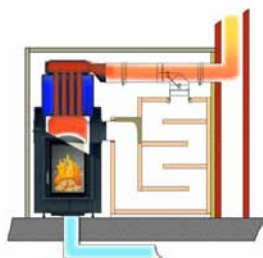
Boiler operation with Moritz's flap
