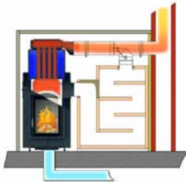
Boiler operation with Moritz's flap
