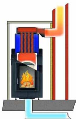
Boiler operation with direct connection
