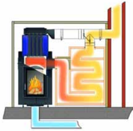
Heat storage mode with Moritz's flap
