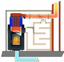
Boiler operation with Moritz's flap
