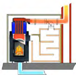
Boiler operation with Moritz's flap
