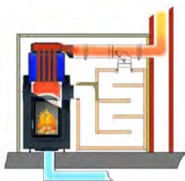
Boiler operation with Moritz's flap
