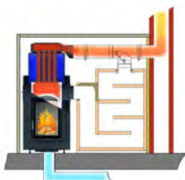
Boiler operation with Moritz's flap
