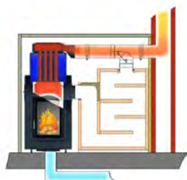
Boiler operation with Moritz's flap
